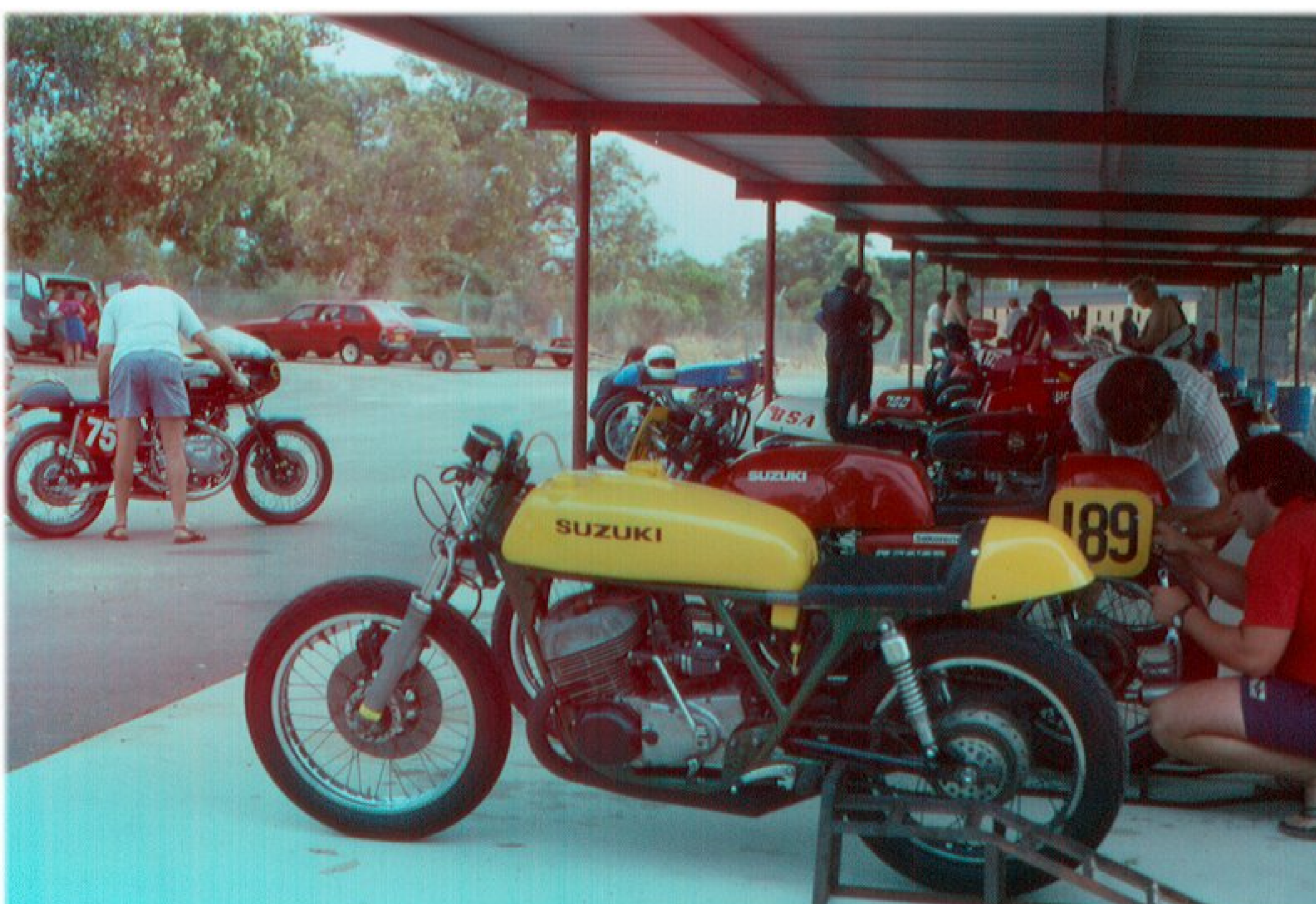
CR750 Honda alloy tank (worth a mint) and a Bromlech 2 into 1 pipe with a Fems racing ignition, went well and was great to ride. Pulled like a train
