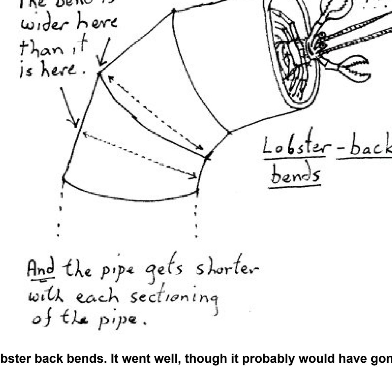
And the pipe gets shorter with each sectioning of the pipe.
