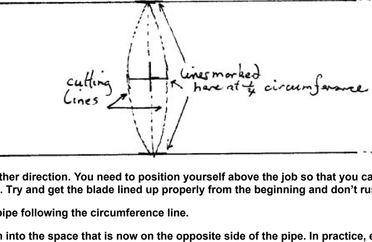
Now you need to decide how big a pie section you need to cut out. Because this depends on how you intend to route your pipe (and its diameter) I can't give you a firm guide on this. I have found that about the depth of a hacksaw blade seems a good place to start for less extreme bends and twice this really rarks the pipe round. I use two bends if I have to come round that sharply.
