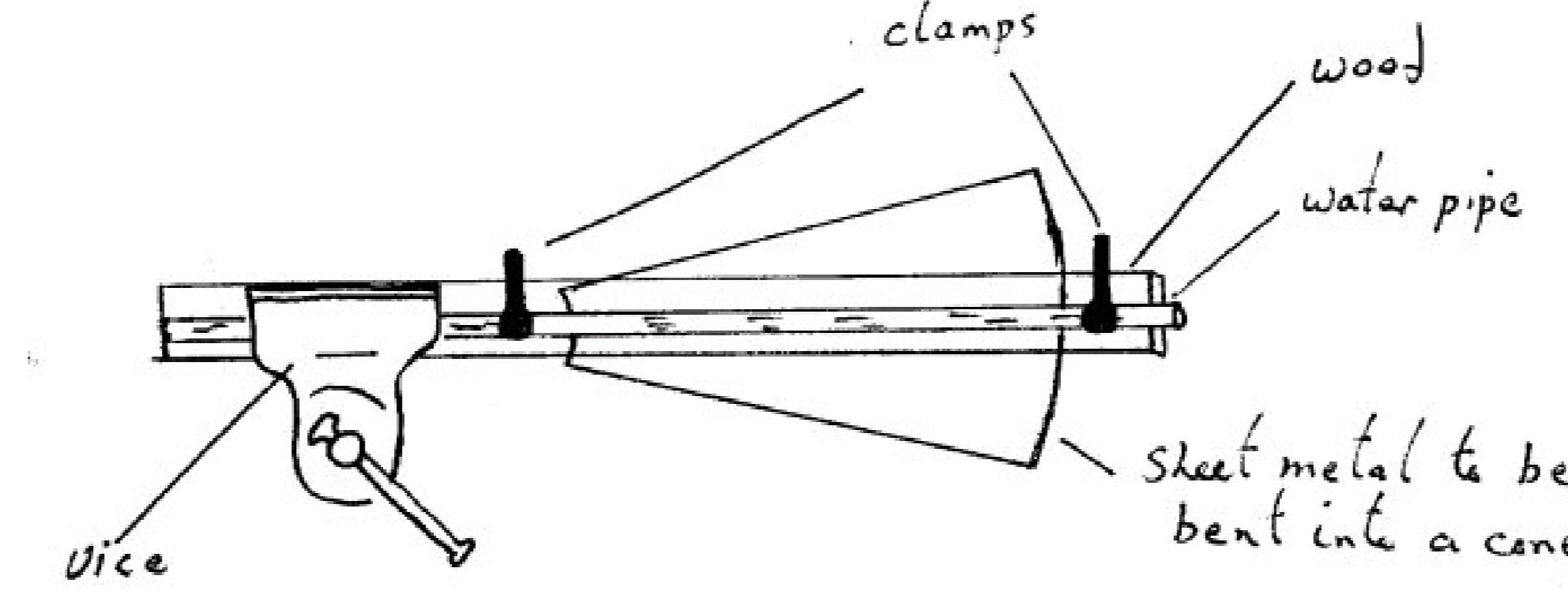
I clamped the wood and the pipe horizontally in the vice, then I slid the piece of metal to be formed between the wood and the pipe, with the smaller end of the cone-to-be at the vice end. The next step was to clamp the pipe and the wood together so that the pipe bisected the metal from end to end.
