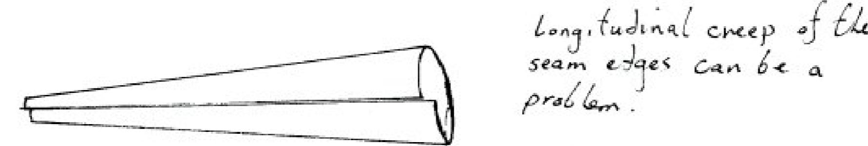
Now, little by little, work the sheet metal around the pipe clamping and unclamping and moving the metal through a wider arc at the larger end. Then reverse the metal so that the small end faces away from the vice, and work the other half round bit by bit.
