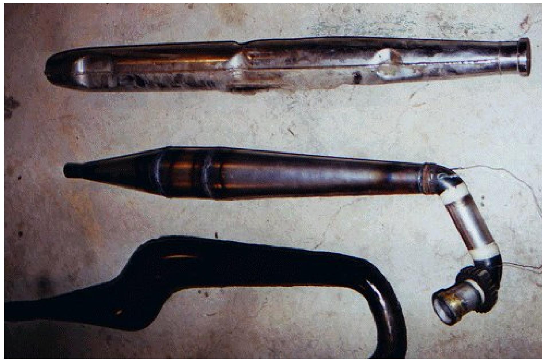
The main advantage to making your own chambers similar to the stock "mufflers" will probably be the weight saving. One of the problems, however, will be that your chambers will scrape on the ground just as the stock items do. Take heart though, they will not be any worse than standard pipes and probably better if you tuck them up well.
