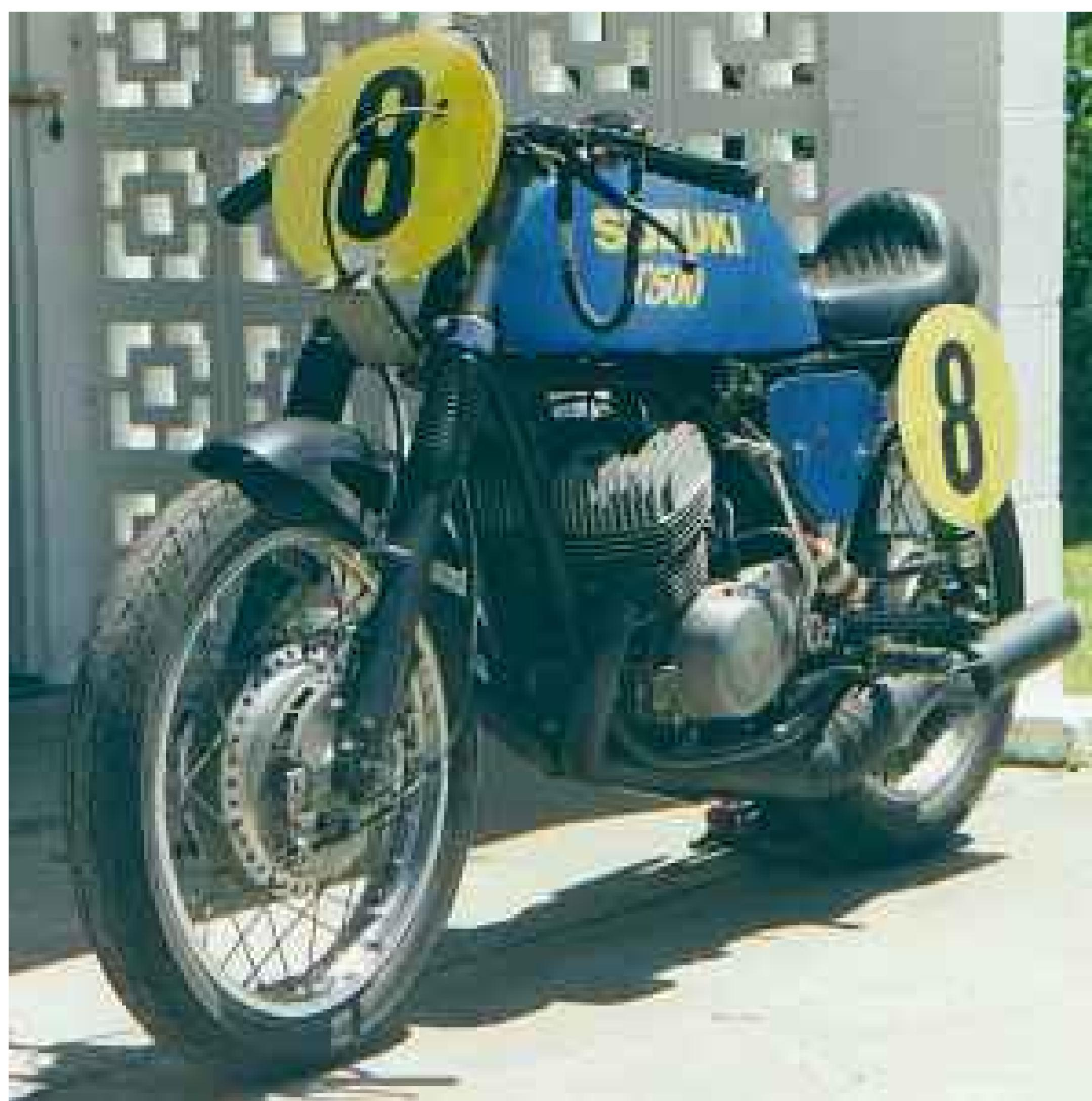
Well, here it is! After five years, three shifts around the country and a few other projects in between. It's finished, it's had a couple of race meetings and it's about to be moth-balled while I head off overseas for a bit. The specs are: Seat, tank, chambers and oil tank by me. Taper roller steering head bearings. RS Honda electronic taco. Forks from a GT 550 disc brake model. GT 550/750 quad shoe front brake. Brake cable balance box by me.
