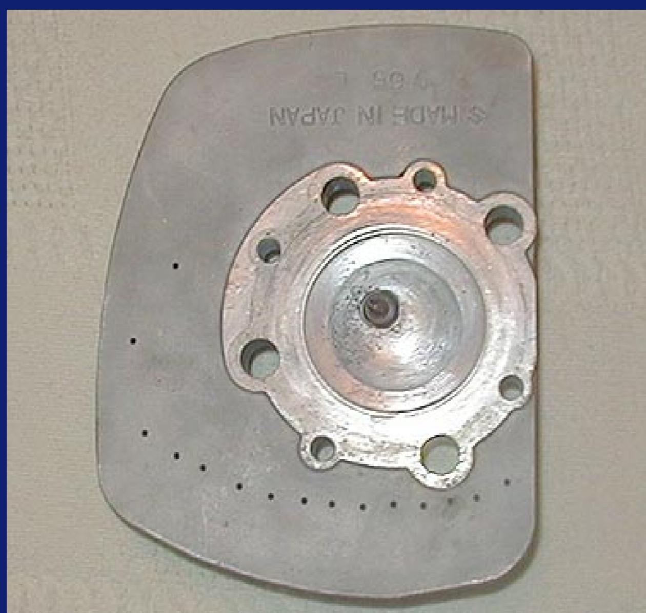
They are welded and then the squish are is machined in. They offer quite a boost in midrange when highend pipes and porting are used. Not as good as TR heads but quite an improvement.
