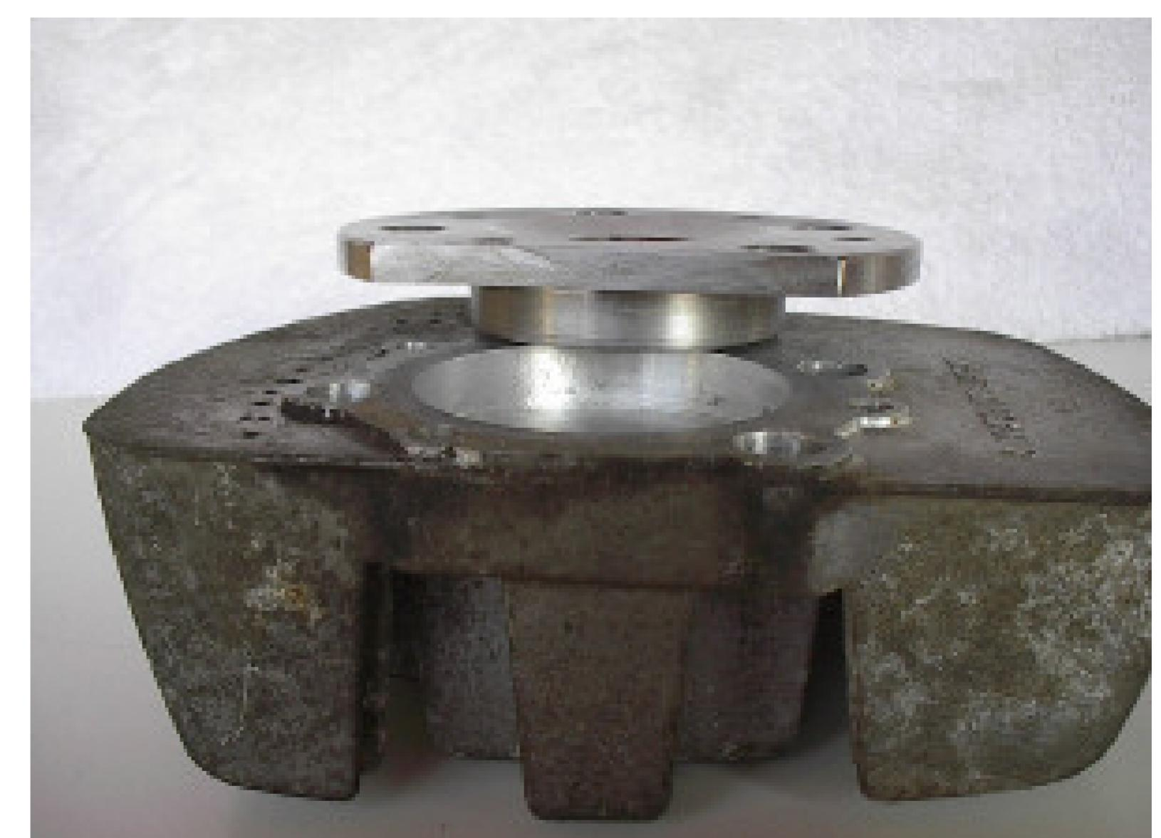
A unique and inventive way to deal with the problem of cracked heads and getting squish heads out of a standard head.
