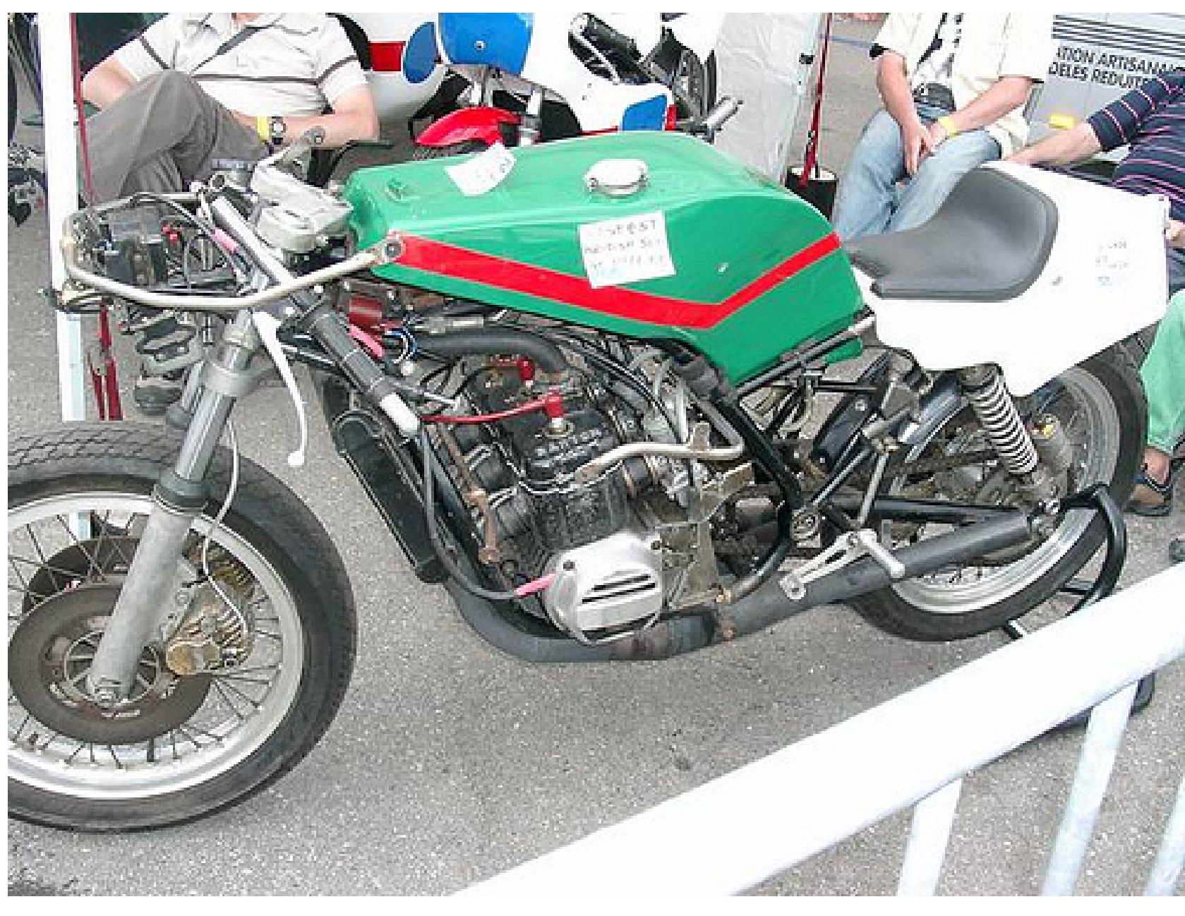
Barton Suzuki 500cc triple on GT380 base with spondon frame also known as Sparton
