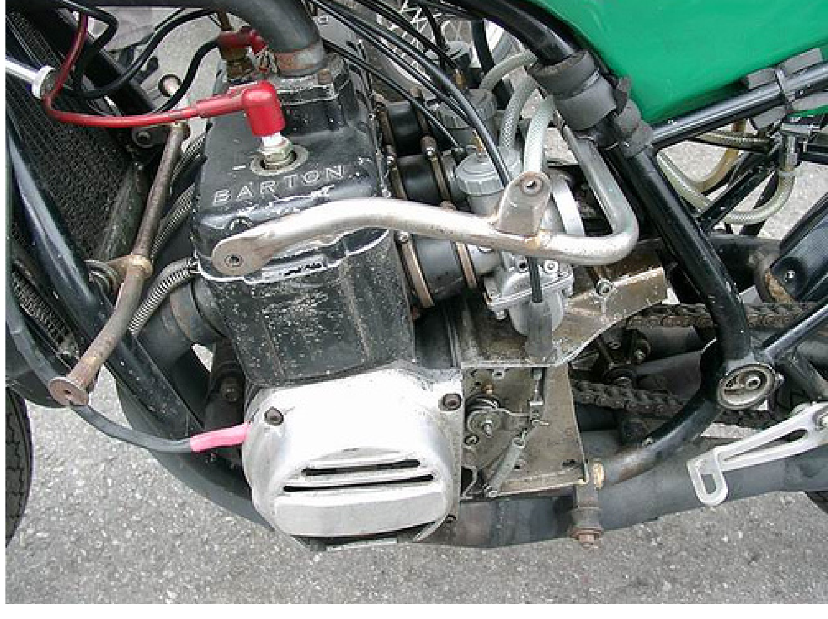
Barton Suzuki 500cc triple on GT380 base with spondon frame also known as Sparton
