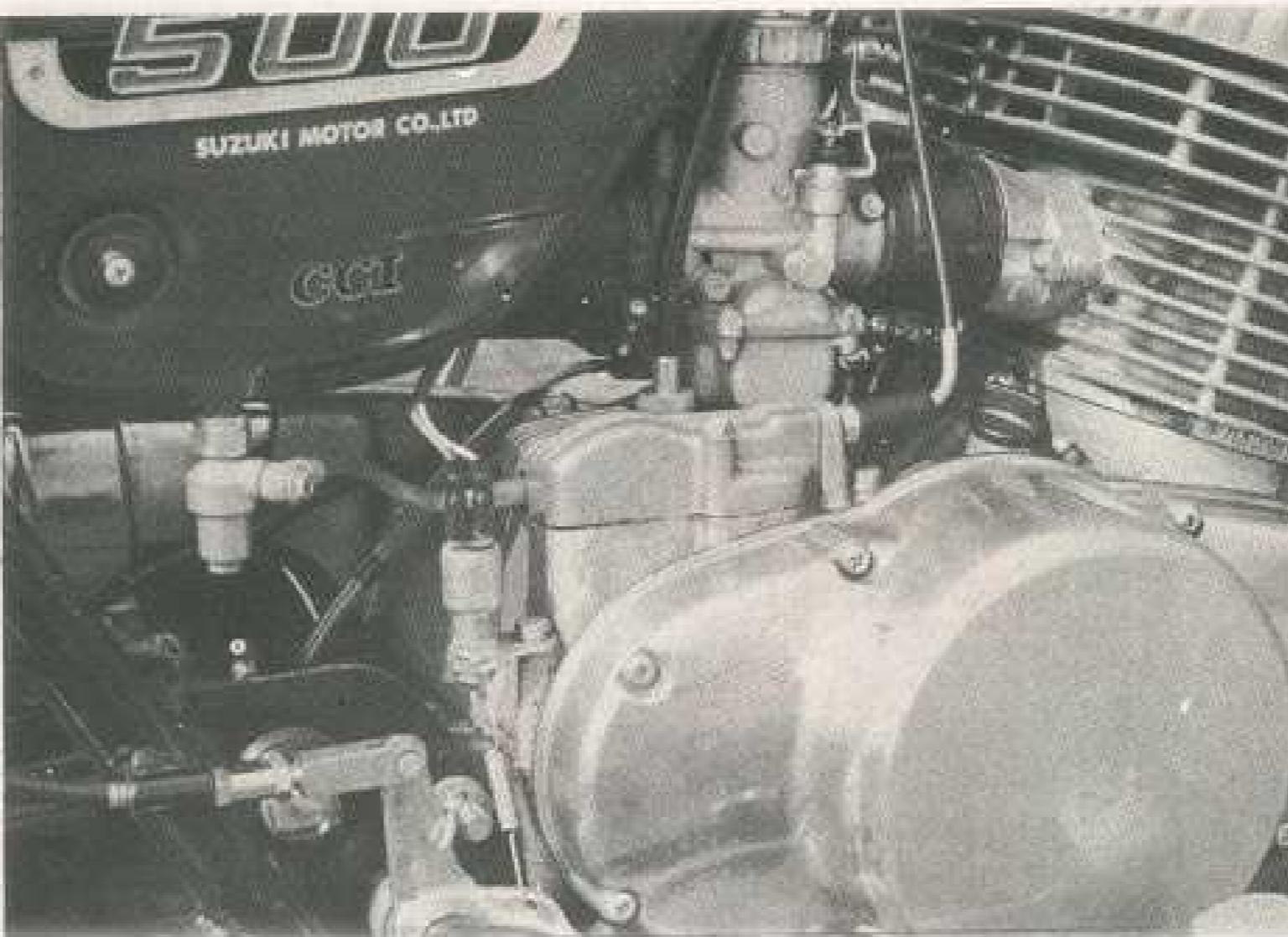
Above: "The Suzuki positive feed system is much more efficient in its use of lubricant than the Yamaha or Kawasaki variants." Below: Very neat, practical control cluster on the left side; and the guide for rear brake-lining wear
