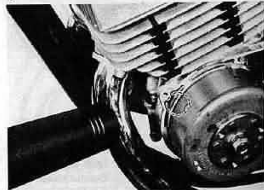
Fig. 9-10 Timing marks on flywheel and crankcase
