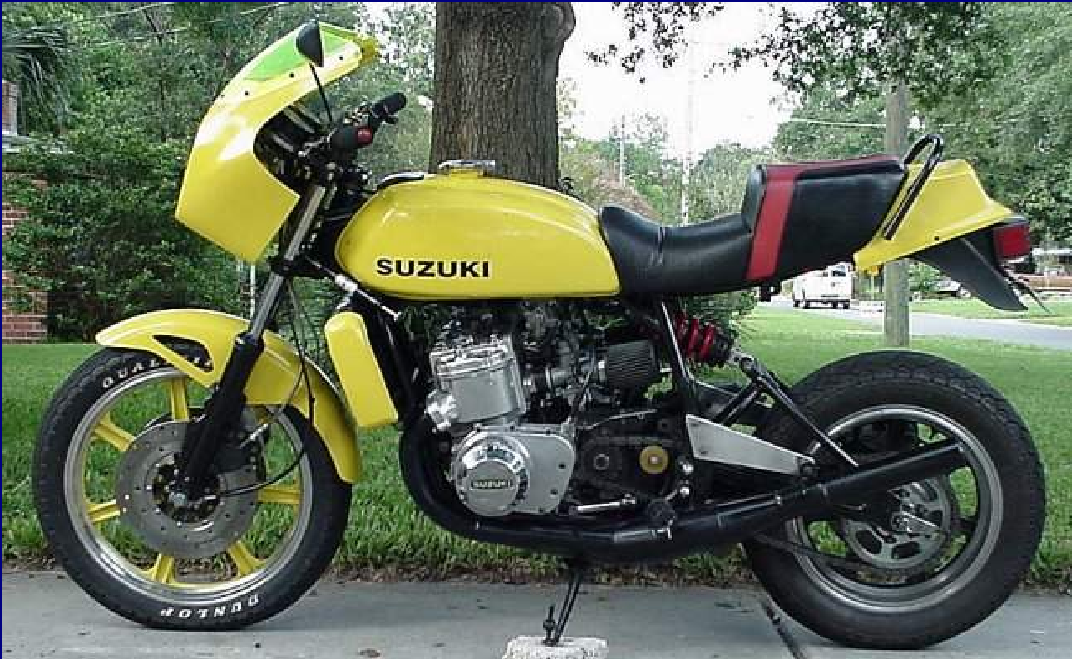
1973 GT750 Suzuki , 1mil over bore , Bassani chambers, clipons, modified ports and carbs, home made swing arm, drilled disks. front stock, rear GS 650, Grimica calipers front , Grimica master rear, cut down Yamaha FJ650 fairing, Kawa 550 seat, oil tank a VW window washer reservor - it and the battery under the seat, Barnett clutch, the frame lightened and braced rear pipe supports removed and lighter ones made. She's lighter and faster but a bit loud. (Editor: and special and unique. Thanks Dave.)
