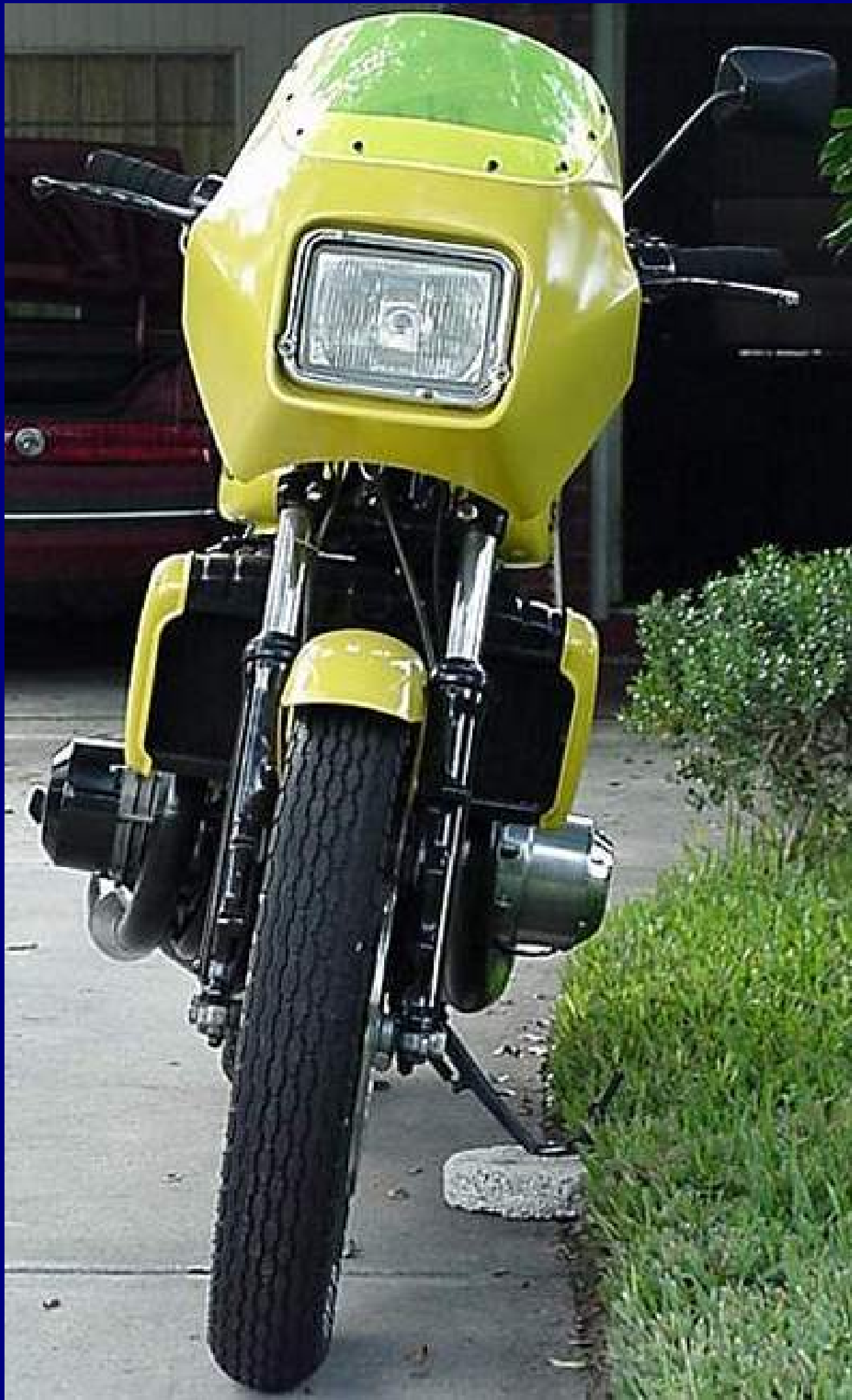
1973 GT750 Suzuki , 1mil over bore , Bassani chambers, clipons, modified ports and carbs, home made swing arm, drilled disks. front stock, rear GS 650, Grimica calipers front , Grimica master rear, cut down Yamaha FJ650 fairing, Kawa 550 seat, oil tank a VW window washer reservor - it and the battery under the seat, Barnett clutch, the frame lightened and braced rear pipe supports removed and lighter ones made. She's lighter and faster but a bit loud. (Editor: and special and unique. Thanks Dave.)
