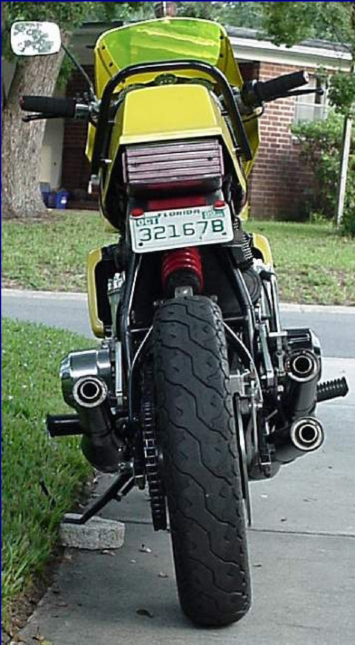
1973 GT750 Suzuki , 1mil over bore , Bassani chambers, clipons, modified ports and carbs, home made swing arm, drilled disks. front stock, rear GS 650, Grimica calipers front , Grimica master rear, cut down Yamaha FJ650 fairing, Kawa 550 seat, oil tank a VW window washer reservor - it and the battery under the seat, Barnett clutch, the frame lightened and braced rear pipe supports removed and lighter ones made. She's lighter and faster but a bit loud. (Editor: and special and unique. Thanks Dave.)
