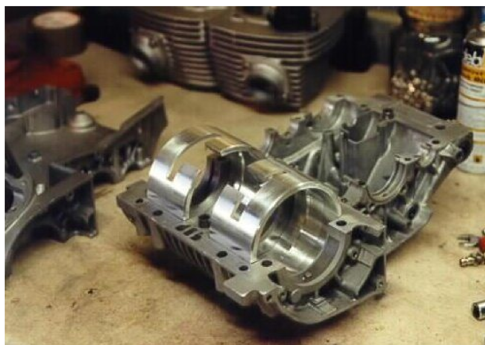
Stuffers fitted in the machined crankcase
