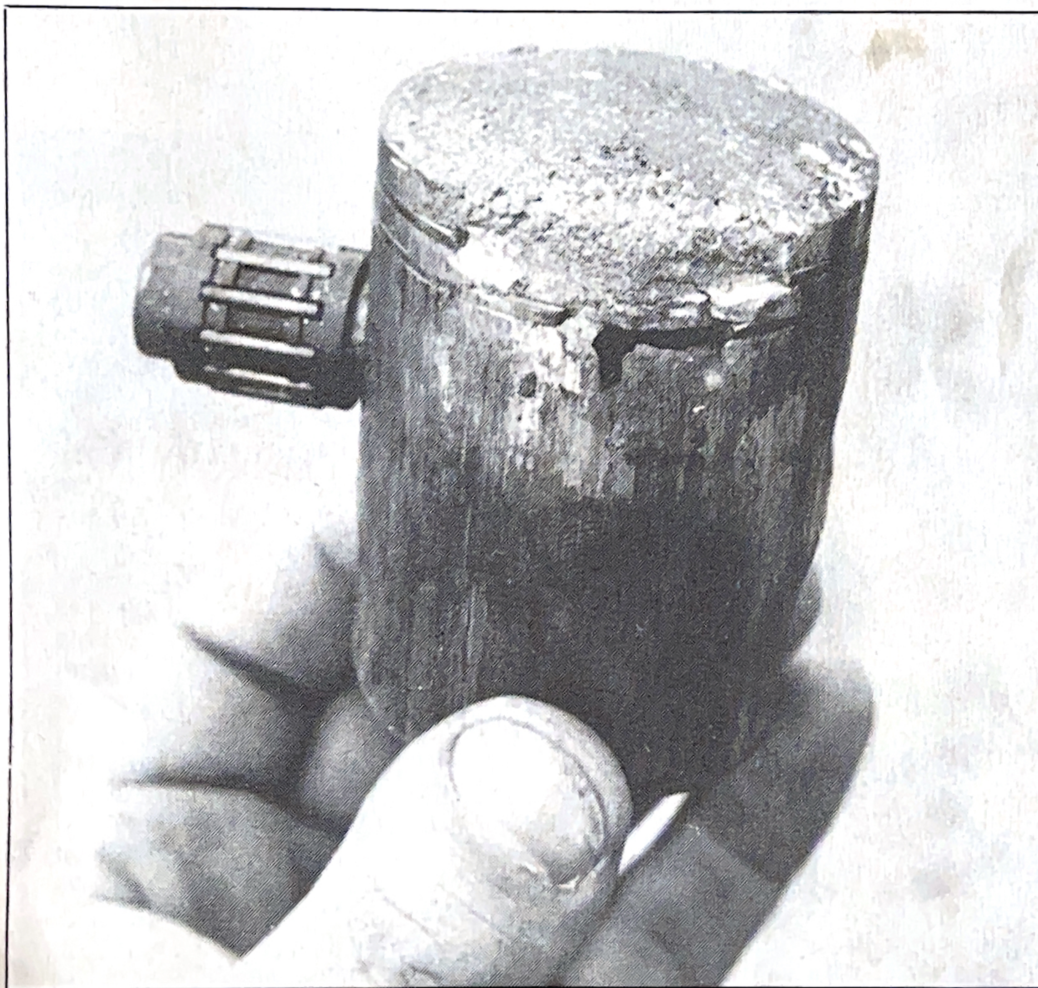
Damaged piston after the Suzuki self-destructed during the test due to a faulty crankshaft. Rider Les Trotter was not displeased – better during a test than five days later in a race.
