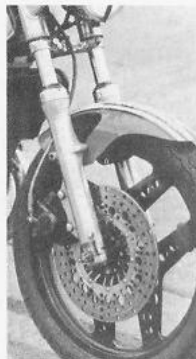
MBX80 wheel carries the severely lightened Suzuki disc and a GSX1100 caliper.
