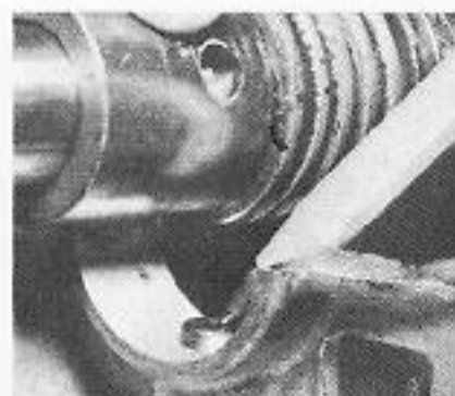
Kickstart shaft bushes are pegged into position. Make sure shaft fits fully into recess.
