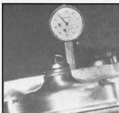
22. Timing must be done with a dial gauge. Centre pot is different to others, and remember that engine turns the 'wrong' way.
