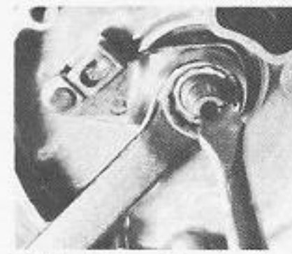
Clutch adjustment is set without the cable being fitted. End float must be just right.
