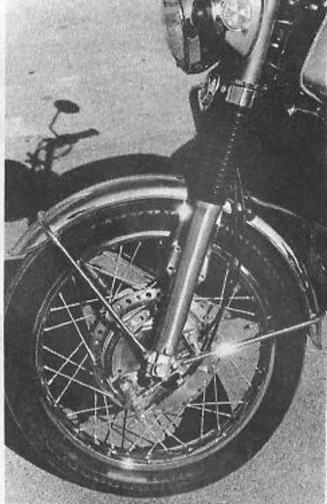
Although the bike is probably the most comfortable machine now offered for sale, it is our opinion the front fork springs are not adequate. It would be better to use a stiffer spring. Rebound damping was fair.
