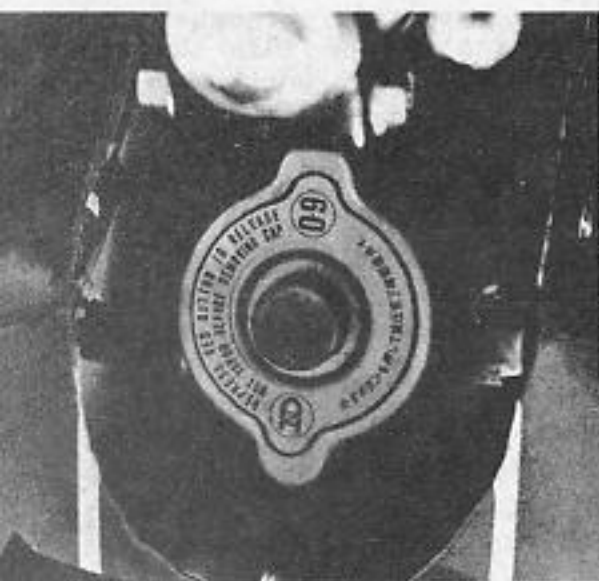
Filler cap for radiator is concealed beneath this flip-up panel at the front of the gas tank. Radiator capacity is 4.5 quarts, and an electrically operated fan assures that temperatures remain within reason.
