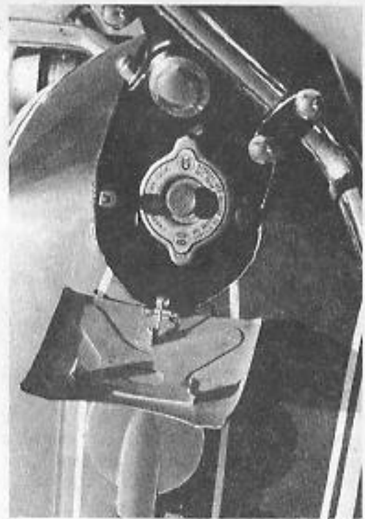
Located under a spring-loaded trap door just ahead of the gas cap is the water filler. We recommend filling the system with anti-freeze and not water, to prevent corrosion in the all aluminum engine.
