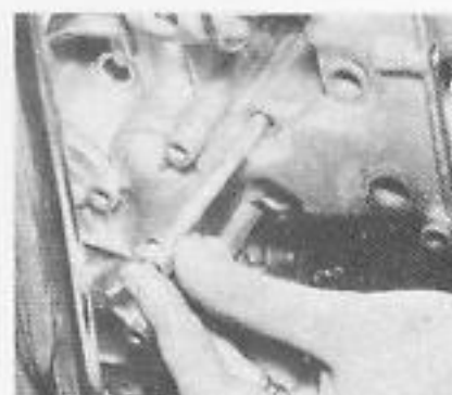
The vital crankcase bolt 13. This bolt must be smothered in Suzuki Bond No 4 to ...
