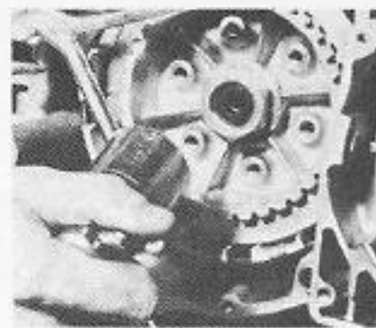
Special clutch holding tool is needed to make sure that the centre nut is done up tight.
