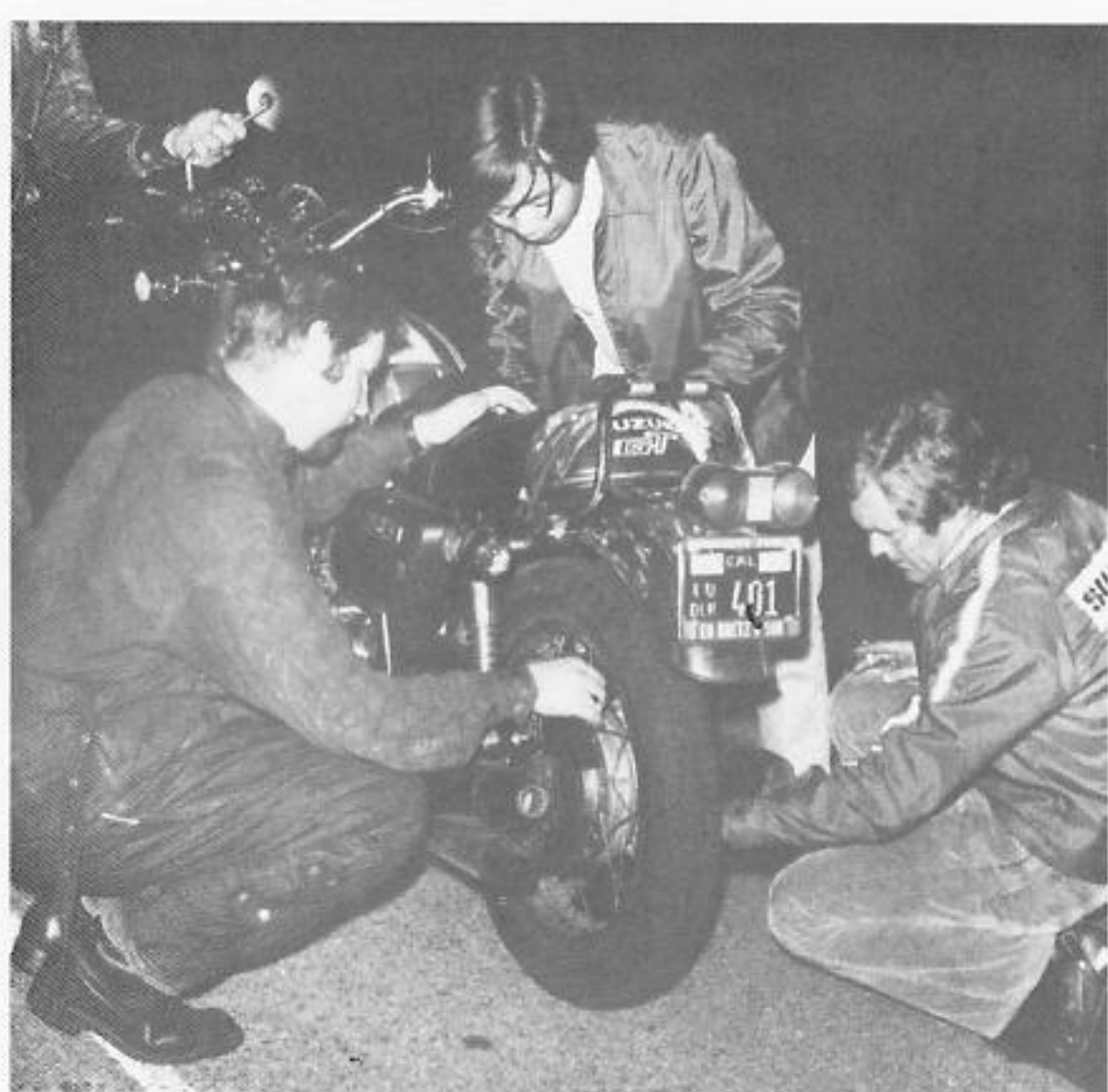
Top: Testing was not without any incidents. Spokes in rear wheel of 750 got so loose wheel wobbled. Left: Double-bulb taillight is good feature, industry should take note. Bottom: Adding oil to any of the three is a chore. Filler neck on oil tank is small, recessed too far.
