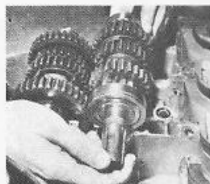
When shafts are fitted give them a spin to make sure that they are mounted correctly.
