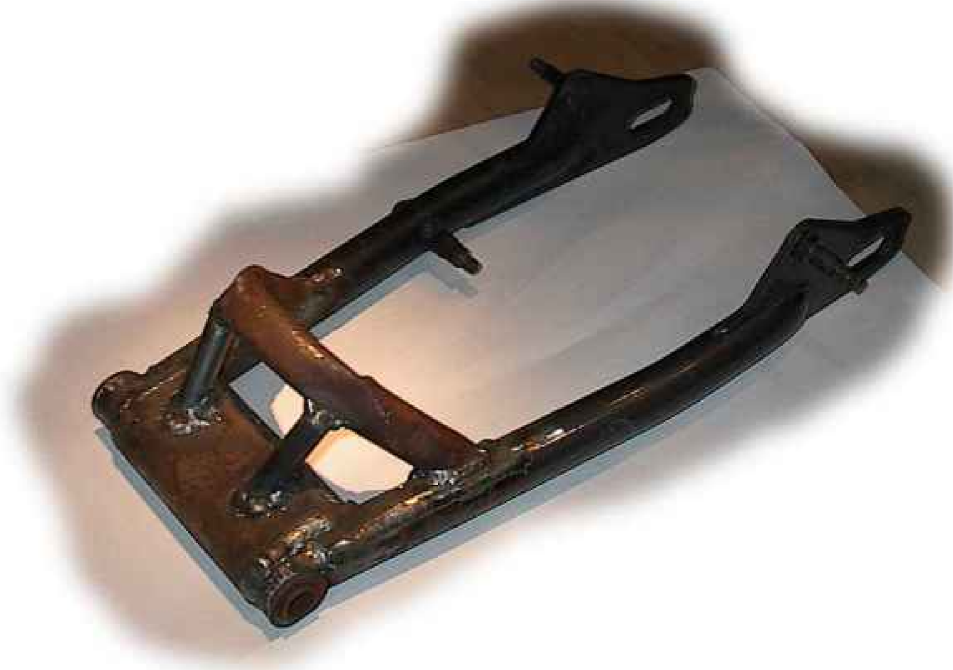
Shortened and strengthened swingarm
