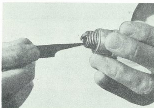
Fig. 10-2-16 Removing carbon deposits
