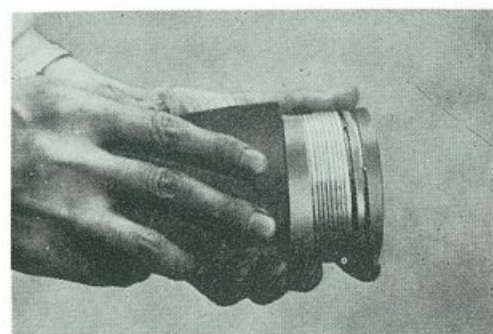
Fig. 8-10-4 Polishing piston surface
