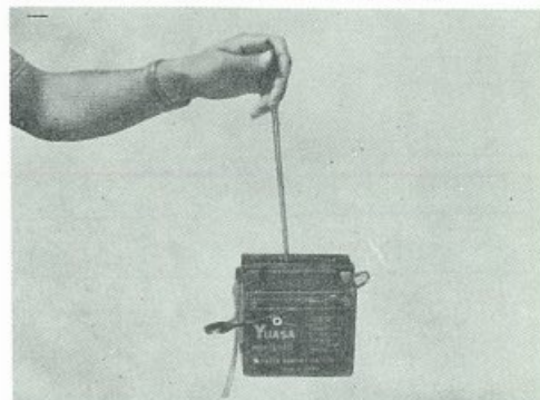
Fig. 10-6-4 Measuring solution temperature
