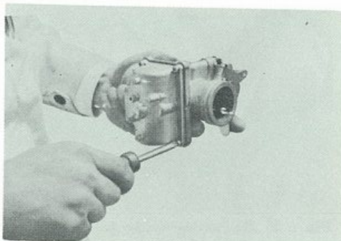
Fig. 8-25-16 Loosening four fitting screws
