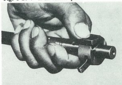
Fig. 8-24-5 Check kick starter pawl roller operation
