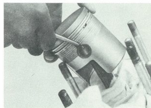
Fig. 8-8-1 Removing piston pin circlip
