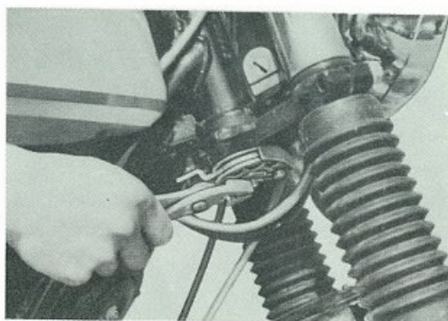
Fig. 9-5-1 Removing damper pin
