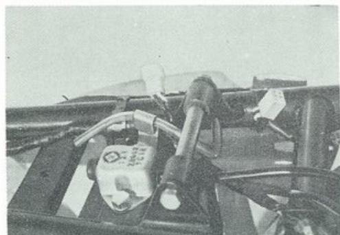
Fig. 9-4-4 Checking oil breather pipe
