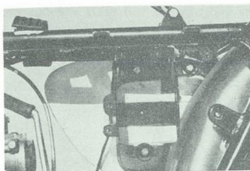
Fig. 9-4-2 Oil tank fitting bolts
