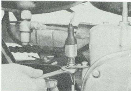
Fig. 8-3-7 Removing brake lamp switch
