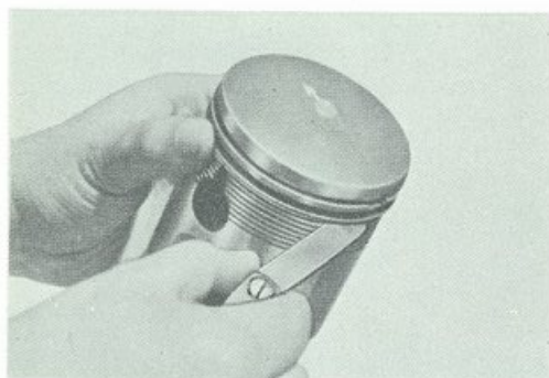
Fig. 8-11-4 Checking side clearance
